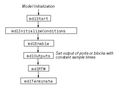
If the S-function resides in a conditionally executed subsystem, it is possible for the generated code to interleave calls to mdlInitializeConditions and mdlStart. Consider the following Simulink model sfcndemo\_enablesub.
