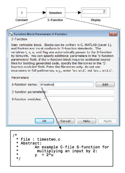
In this example, the model contains an S-Function block that references an instance of the C MEX file for the S-function timestwo.c.
