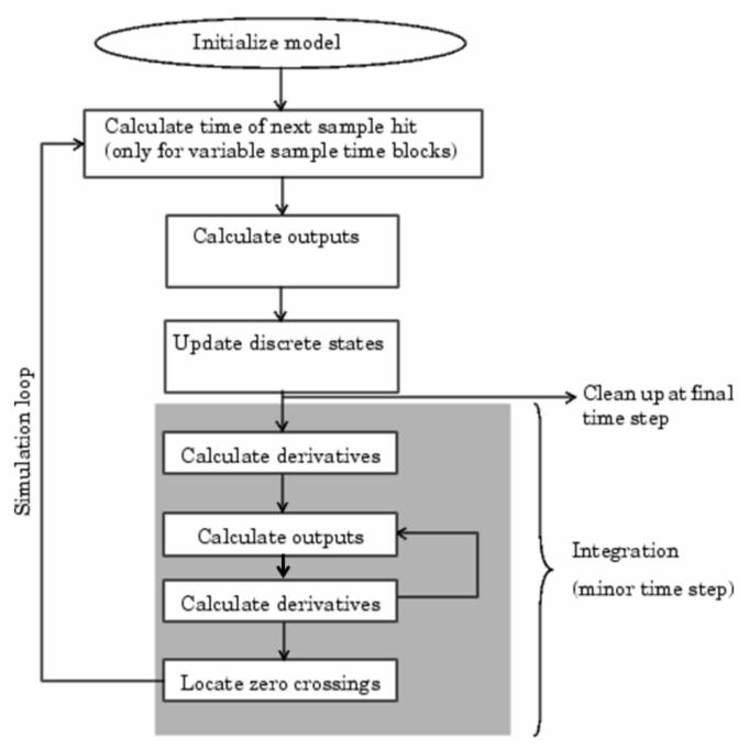
How the Simulink® Engine Performs Simulation
