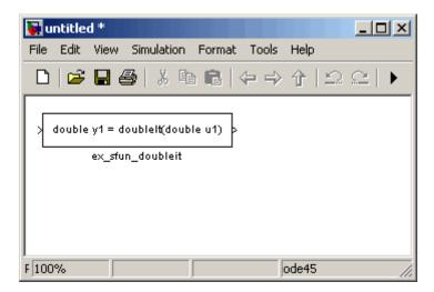
The following Simulink model demonstrates that the C MEX S-function produced by the Legacy Code Tool behaves like the C function doubleIt. In
